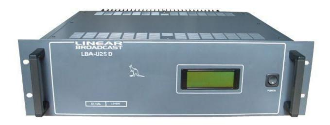
The Linear Broadcast 25 watt COFDM broadcast amplifier is a reliable, conservatively rated unit and is fully self contained in a 3RU powder coated rack case. It is fitted with front panel metering of output power and supply voltages. It accepts a single or multi channel low level RF input from a COFDM modulator and outputs up to 25 Watts in the UHF television band.
